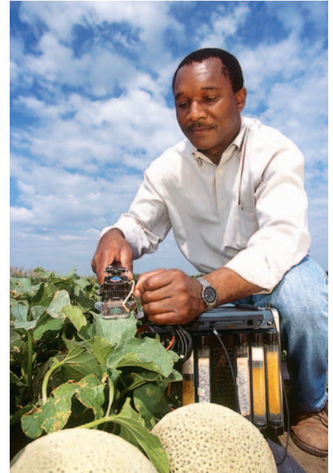
John Jifon, a plant physiologist at Texas A&M University Experiment Station, measures photosynthetic activity of plants sprayed with potassium for comparison to that of nonsprayed plants.
